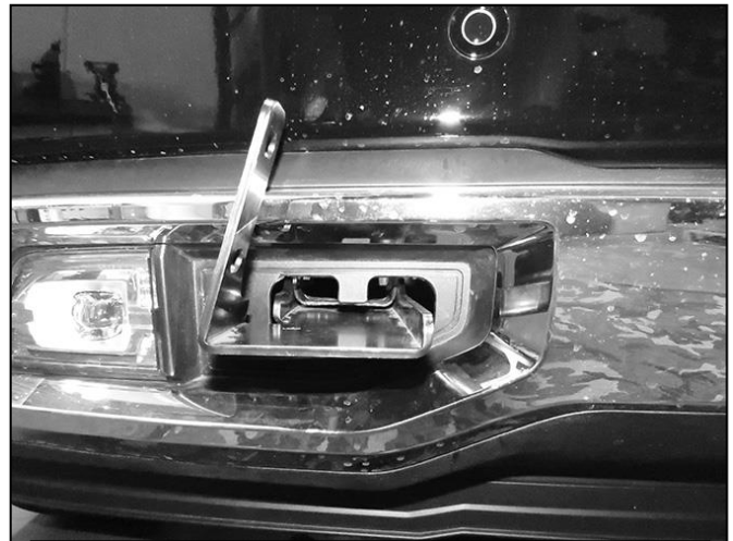
(Fig 11) Passenger/right side Bracket installed
