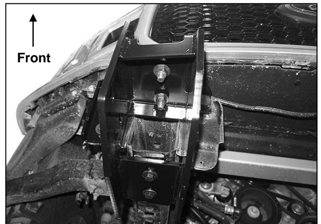
(Fig 6) Passenger/right Frame Bracket attached to bottom of frame and Double Nut Plate
