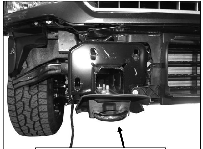
(Fig 4) Remove the tow hooks and plastic seals, (if equipped)
