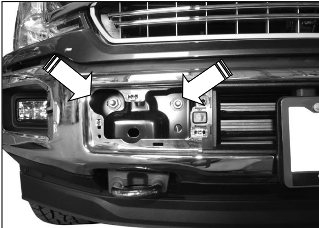
(Fig 3) Remove (2) factory hex nuts from each side
