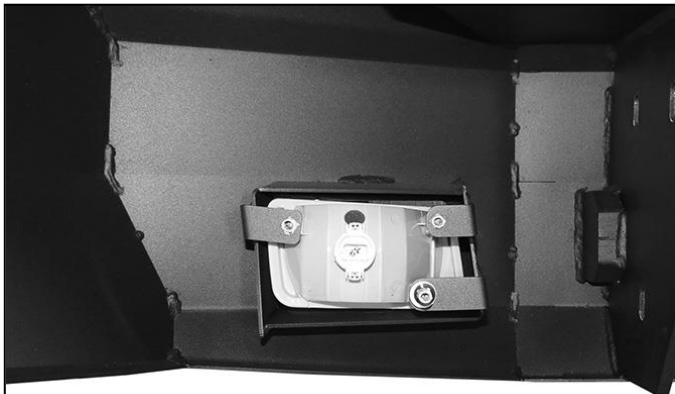
(Fig 14) Driver/left side of Bumper attached to Winch Tray Bracket Assembly
