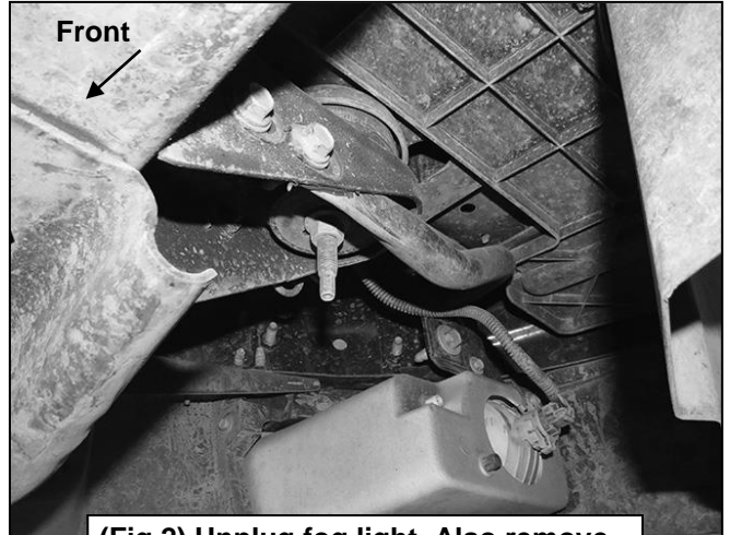
(Fig 2) Unplug fog light. Also remove bumper support from side of frame (arrow). Passenger/right side pictured
