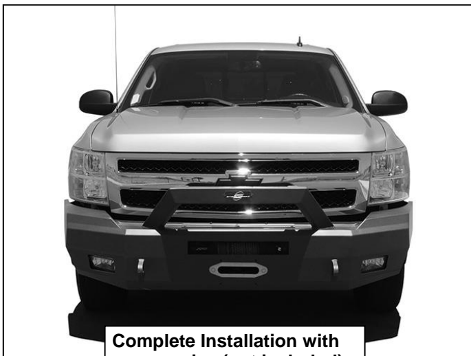
(Fig 16) Remove (3) screws from lights. Adjust tabs on Bumper if necessary to line up with light. Reuse screws to attach light to tabs on Bumper.
