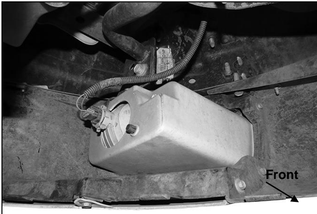
(Fig 1) Unplug fog light and wiring harness. Also remove bumper support from side of frame (not pictured). Driver/left side pictured
