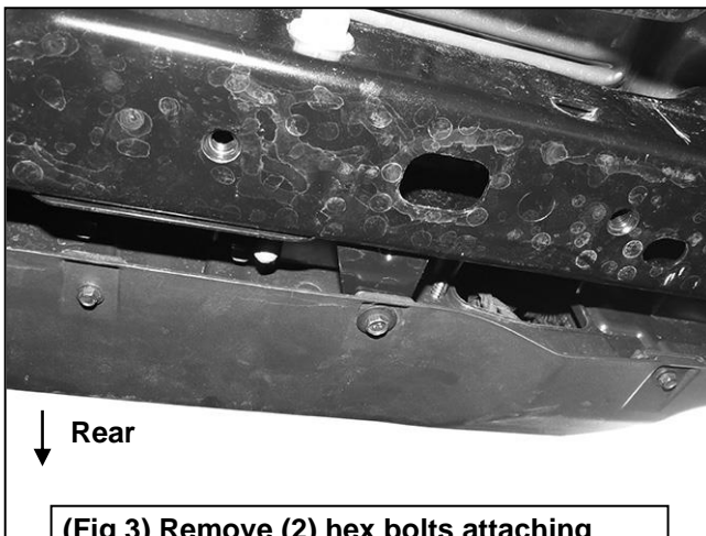
(Fig 3) Remove (2) hex bolts attaching bottom of bumper to frame cross member
