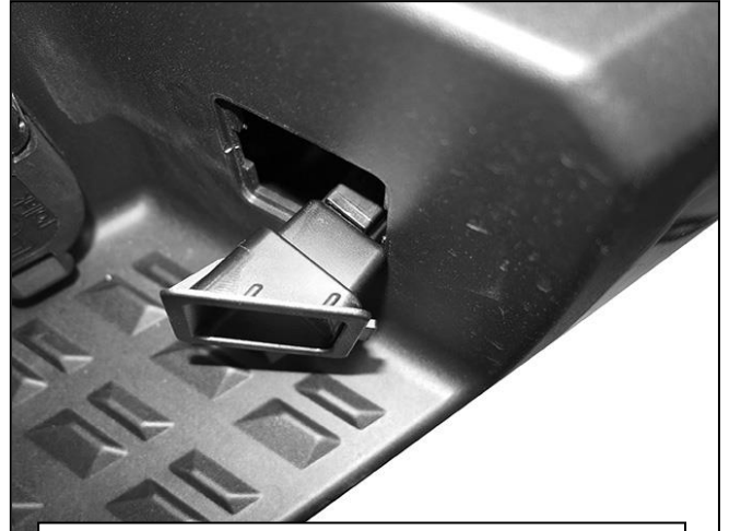
(Fig 2) Unplug license plate lights and trailer connector. Remove lights and connector
