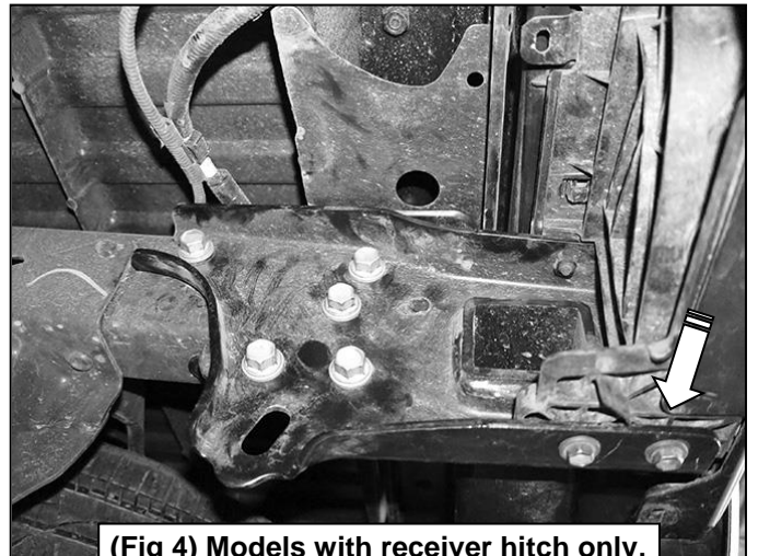
(Fig 4) Models with receiver hitch only, remove hex bolts attaching bumper to bottom of receiver hitch (arrow).
