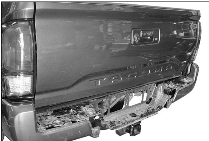
(Fig 3) Models with receiver hitch only, remove plastic cover from top of bumper to access hex bolts attaching bumper to top of receiver hitch
