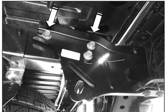
(Fig 2) Models without receiver hitch only, remove (3) factory hex bolts (arrows) attaching brackets to both sides of frame and slide off bumper assembly
