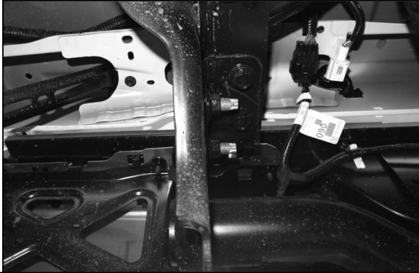
(Fig 1) Unplug and remove 7-wire trailer plug, unplug license plate lights and sensors if equipped
