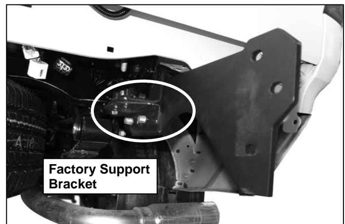
(Fig 9) Attach Mounting Bracket to the frame and support bracket. Note: the mounting bracket mounts to the outside of the receiver hitch for models with a receiver hitch.
