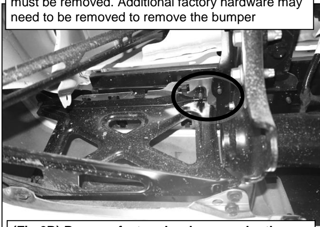
(Fig 6B) Remove factory hardware under the plastic pieces.
