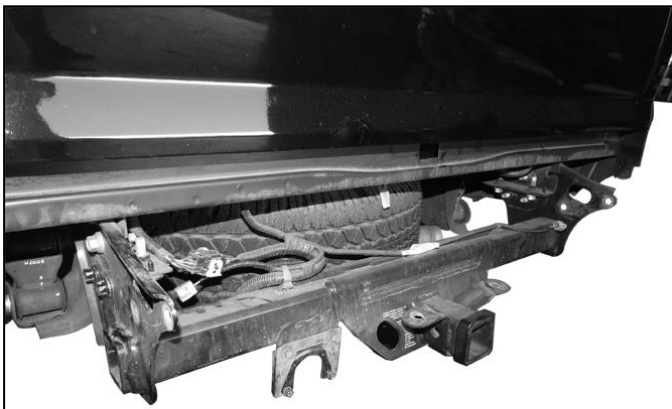
(Fig 5) Models with receiver hitch only, remove bumper but leave receiver hitch attached
