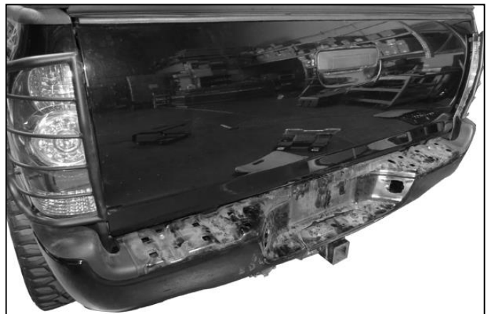
(Fig 2) Models with receiver hitch only, remove plastic cover from top of bumper to access hex bolts attaching bumper to top of receiver hitch
