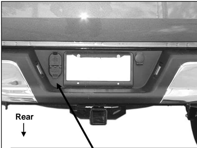
(Fig 1) Unplug and remove 7-wire trailer plug
