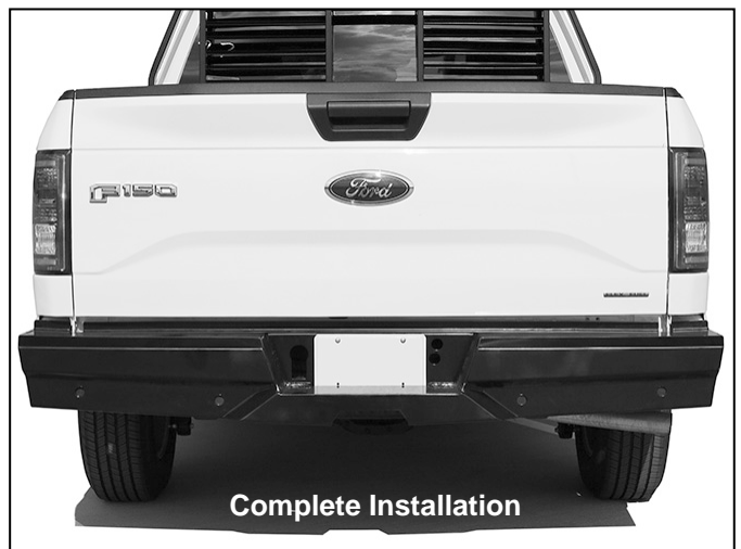
(Fig 15) Push plastic plugs into holes for license plate
