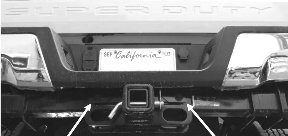
(Fig 1) Remove the two bolts securing the bumper step to the hitch.
