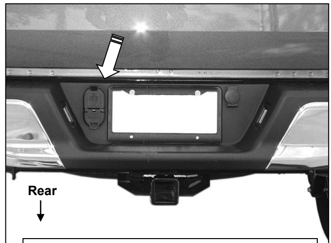
(Fig 2) Unplug and remove 7-wire trailer plug
