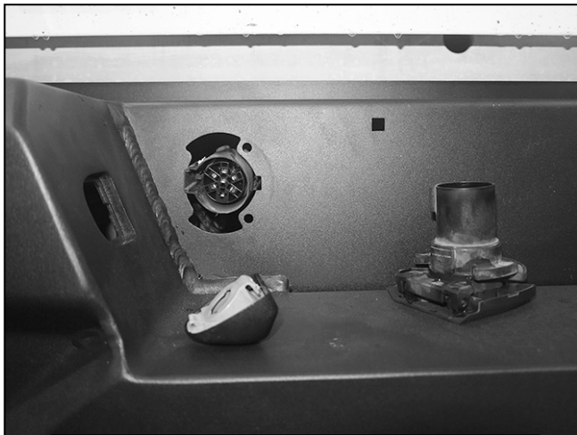
(Fig 11) Install license plate lights, trailer plug and spare tire access lock
