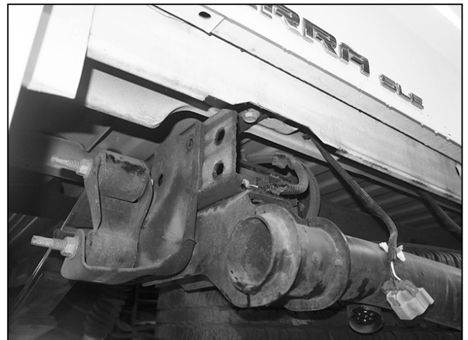
(Fig 4) Unplug wiring harness leading to bumper. Slide complete bumper assembly out of frame
