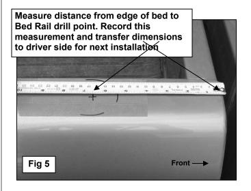
Measure distance from edge of bed (side) to Bed Rail center drill point. Record this measurement and transfer dimensions to the rear mounting location and to the driver side for next installation
