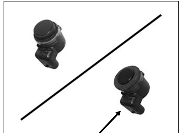
(Fig 6) Remove silicone seal from sensor. Slide large Seal over end of sensor (arrow)
