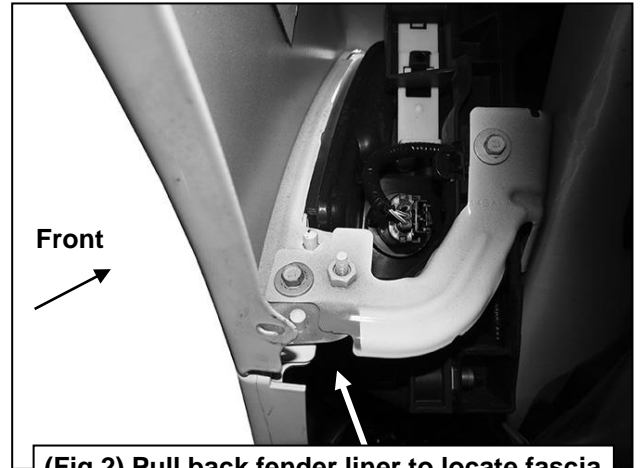
(Fig 2) Pull back fender liner to locate fascia attachment at bottom of front fender
