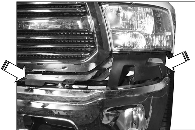
(Fig 3) Remove fascia body panel from top of bumper, (arrows) or 1pc plastic bumper cover
