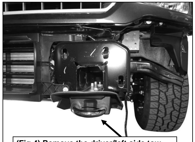
(Fig 4) Remove the driver/left side tow hook and plastic cover, (if equipped)
