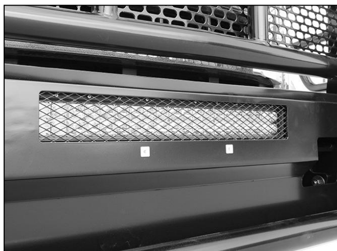
(Fig 14) Push plastic plugs into holes in Bumper for license plate if required. LED bar light pictured installed behind Bumper on non-ecoboost model. LED light installation not recommended on ecoboost models
