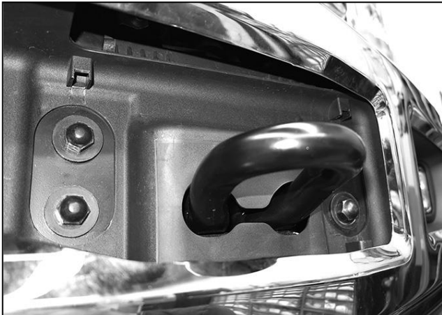
(Fig 6) Remove bumper bolts (driver side pictured)
