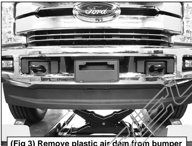
(Fig 3) Remove plastic air dam from bumper
