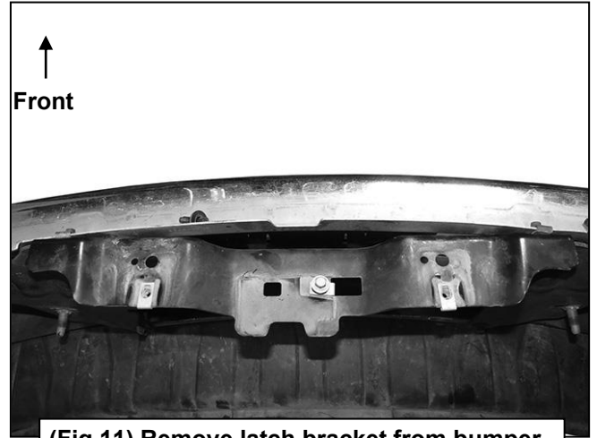
(Fig 11) Remove latch bracket from bumper
