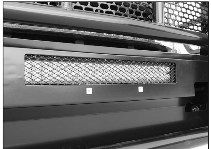
(Fig 18) Push plastic plugs into holes in Bumper for license plate if required. LED bar light pictured installed behind Bumper on non-ecoboost model. LED light installation not recommended on ecoboost models
