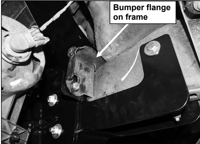
(Fig 15) Attach Outer Support Bracket to flange on frame and center hole in Bumper Bracket
