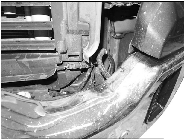
(Fig 5) Disconnect all wire harnesses leading to front bumper
