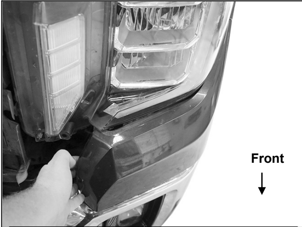
(Fig 3) Pull outward to release plastic fascia body panel from clips. Do not remove, only release inner end to remove grille
