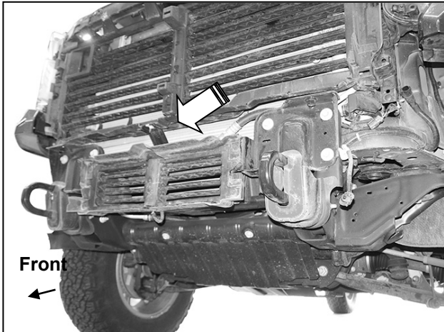
(Fig 8) Remove tow hooks, bumper brackets and shutter assembly (arrow) if equipped
