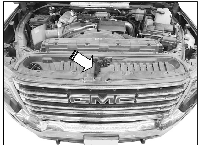
(Fig 2) Open hood. Temporarily remove release handle (arrow). Remove plastic cover from top of grille and radiator
