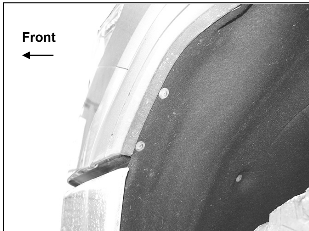
(Fig 1) Release hardware attaching fender liner to back of bumper and fender (driver/left side pictured)
