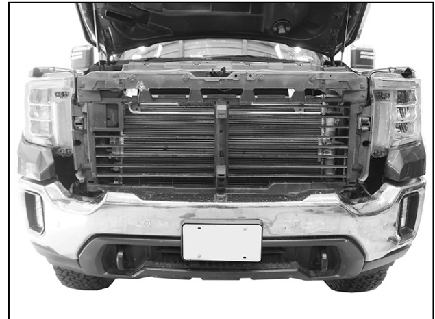
(Fig 4) Disconnect harness to camera (if equipped) and remove grille
