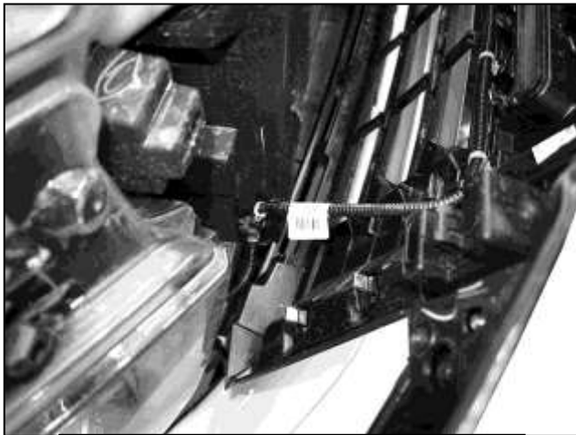
(Fig 5) Disconnect harness to camera (if equipped) and remove grille
