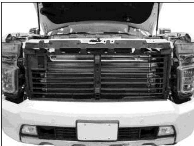
(Fig 7) Grille and fascia removed
