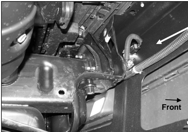
(Fig 1) Unplug sensors, fog lights and move wiring harness away from bumper before removal
