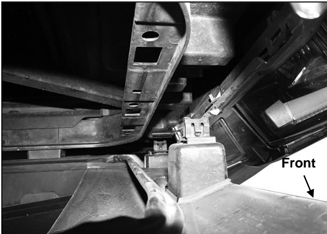
(Fig 3) Firmly pull grille straight out from vehicle
