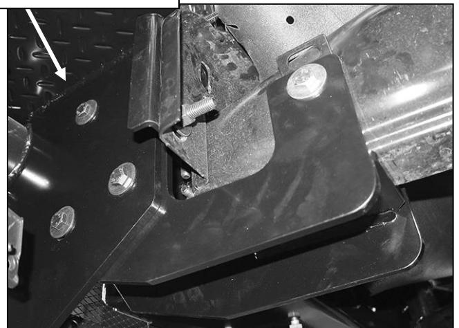
(Fig 15) Driver/left side of Bumper attached to Bracket assembly, (pictured from behind Bumper)
