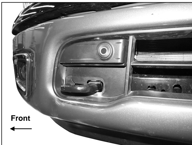
(Fig 1) Passenger/right side equipped with factory tow hook
