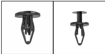
(Fig 5) Example of pop-up style clips: Use a small flat bladed screwdriver to gently pry up the center pin to release clip.
