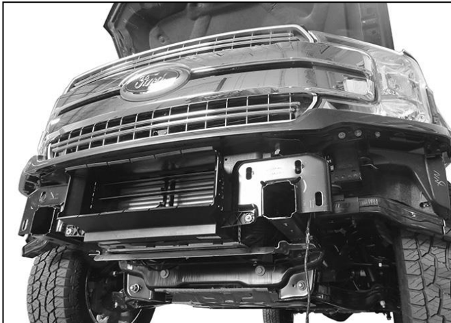
(Fig 18) 2018 models: Remove bumper assembly
