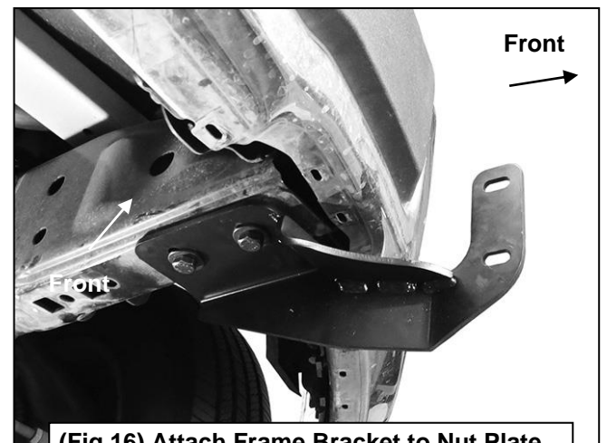
(Fig 16) Attach Frame Bracket to Nut Plate.
