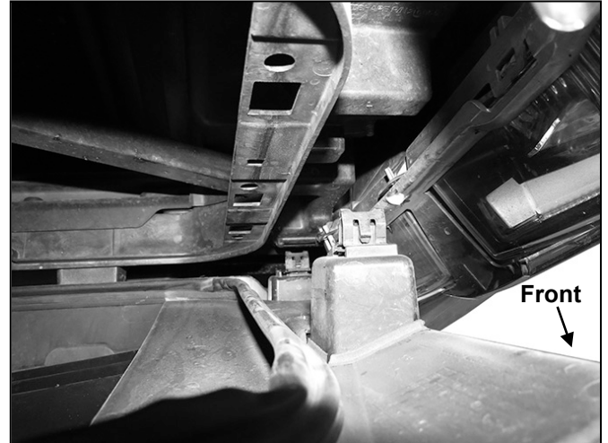
(Fig 4) Firmly pull grille straight out from vehicle
