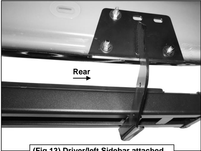
(Fig 13) Driver/left Sidebar attached to rear Mounting Bracket
