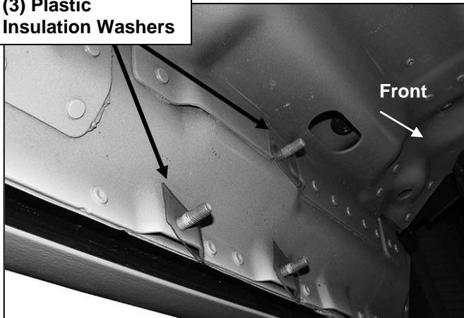
(Fig 1) Driver/Left Front Mounting Location Pictured
