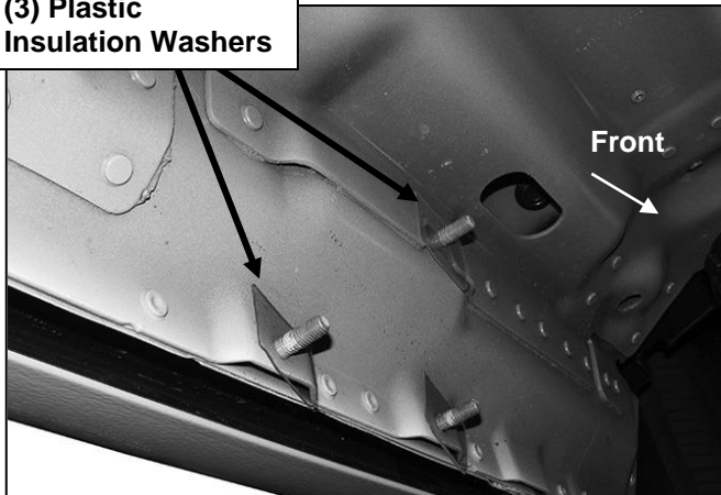
(Fig 1) Driver/Left Front Mounting Location Pictured
