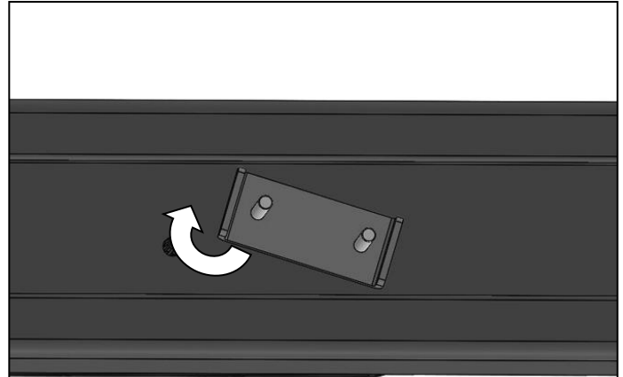
(Fig 6) Insert 8mm Double Bolt Plate through the channel opening in the bottom of the Sidebar
