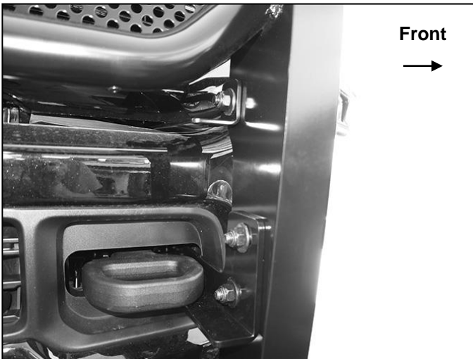
(Fig 14) Attach Grill Guard to outside of driver/left Mounting Brackets
