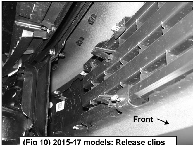
(Fig 10) 2015-17 models: Release clips attaching bumper pad to steel bumper
