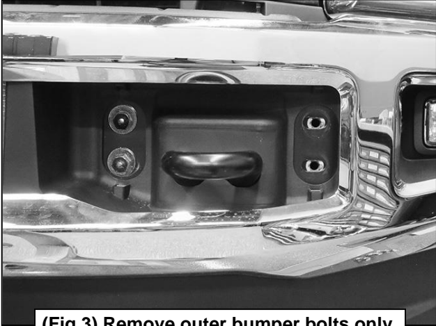
(Fig 3) Remove outer bumper bolts only
