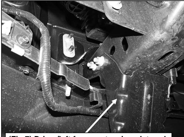
(Fig 7) Driver/left frame extension pictured
