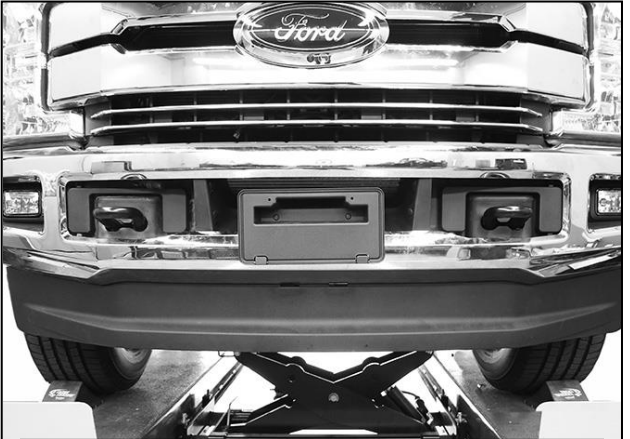
(Fig 6) Remove plastic air dam from bumper
