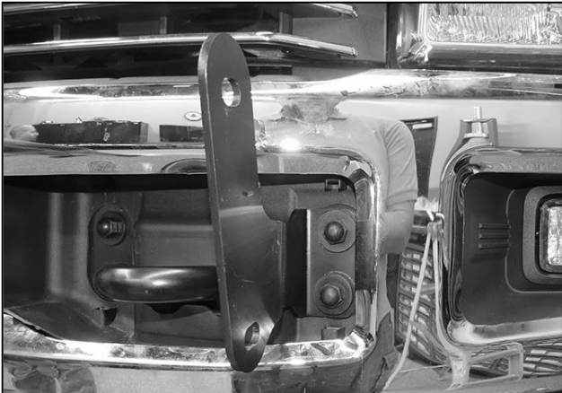
(Fig 5) Reuse factory bumper bolts to attach driver/left Frame Bracket to Spacer and bumper
