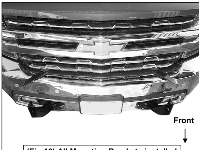
(Fig 16) All Mounting Brackets installed
