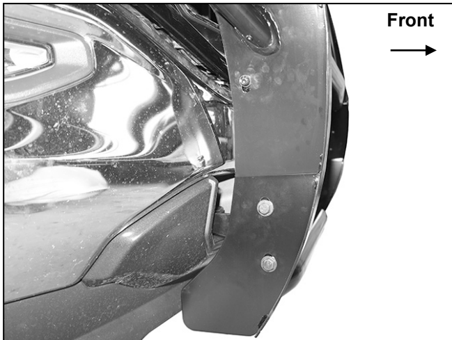
(Fig 26) Grille Guard fully installed
