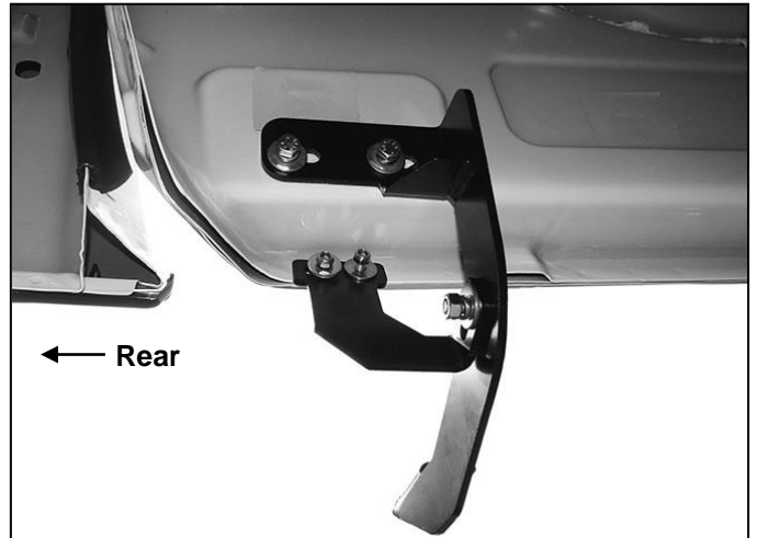
(Fig 16) Driver/Left rear Mounting Bracket assembly
