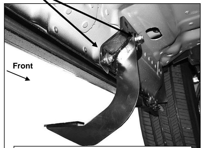
(Fig 4) Driver side front Bracket installation
