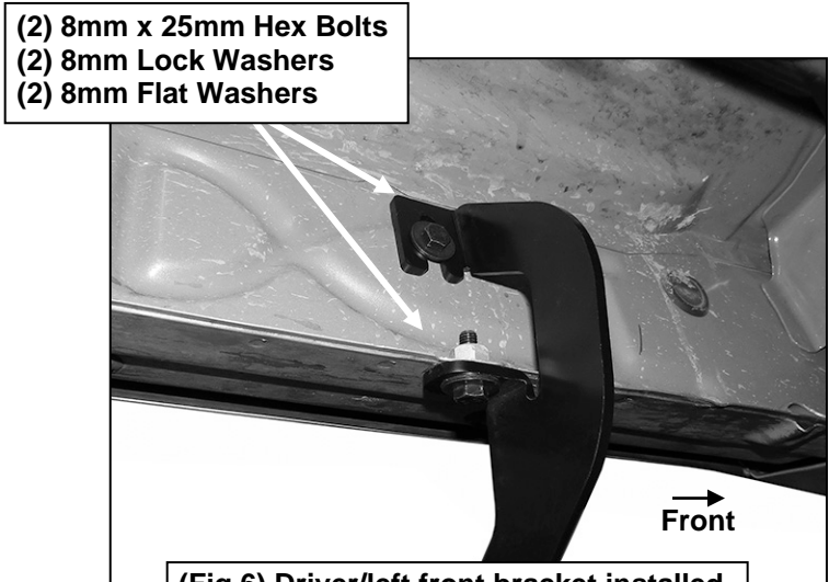
(Fig 6) Driver/left front bracket installed
