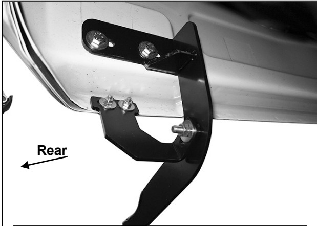
(Fig 16) Driver/Left rear Brackets installed
