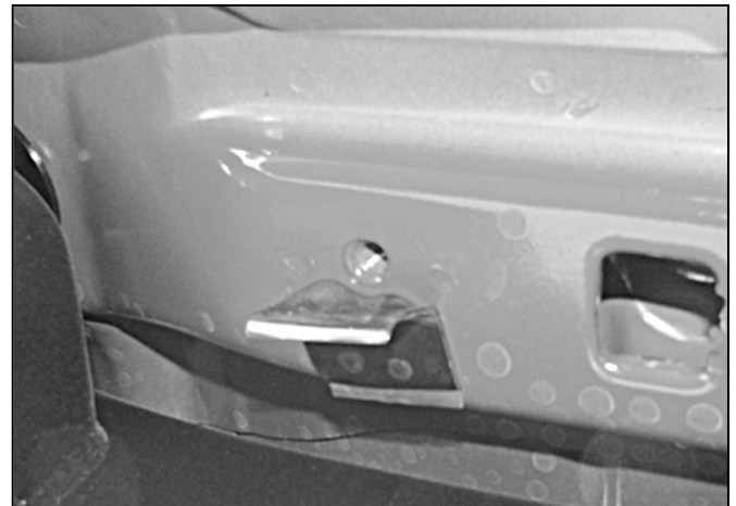
(Fig 2) 8mm threaded hole in floor frame channel (passenger side-front pictured for example)
