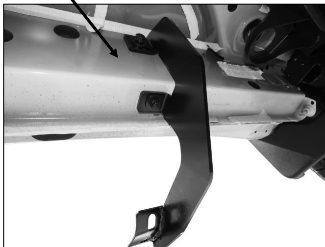
(Fig 4) Driver/left front Bracket installed
