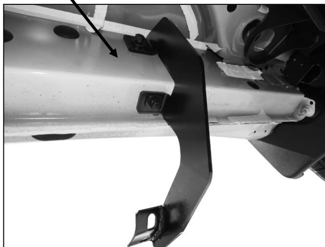
(Fig 4) Driver/left front Bracket installed
