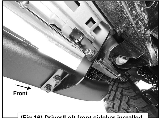
(Fig 16) Driver/Left front sidebar installed
