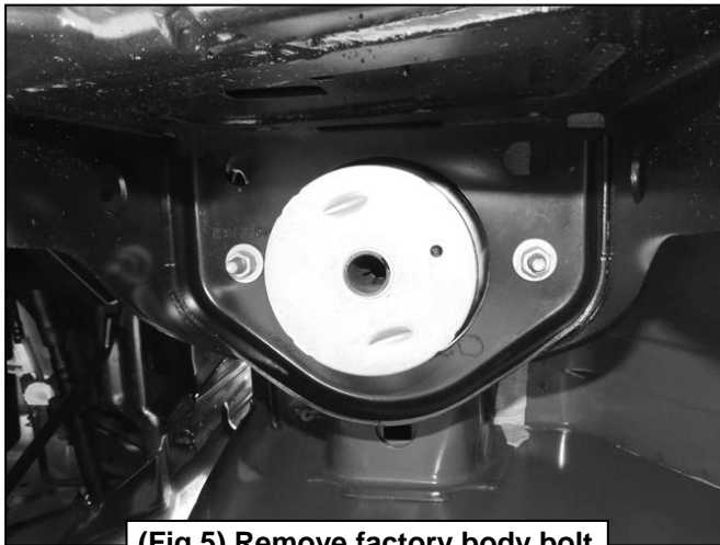
(Fig 5) Remove factory body bolt
