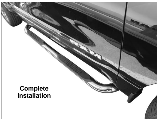
(Fig 12) Driver/left Front Brackets and Sidebar installed
