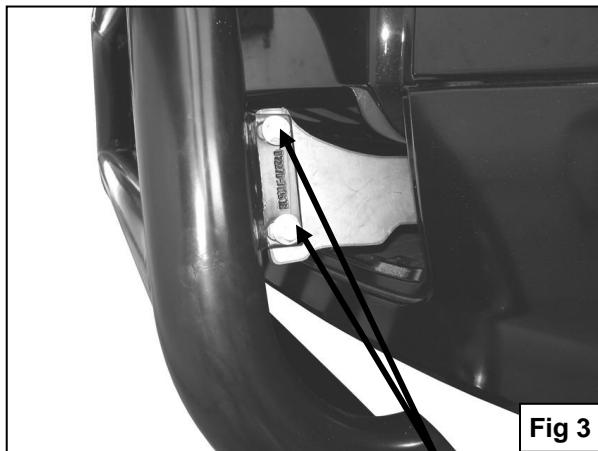
10mm x 35mm Hex Bolts 10mm Lock Washers 10mm Flat Washers 10mm Hex Nuts
