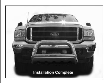
**WARNING!** Do not loosen or remove passenger and driver side bumper mounting bolts at the same time or bumper may move out of alignment or fall off of the vehicle. Only remove the bumper bolts from one side and install one Mounting Bracket at a time.
