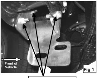
10mm x 35mm Hex Bolts 10mm Lock Washers 10mm Hex Nuts 10mm Flat Washers
