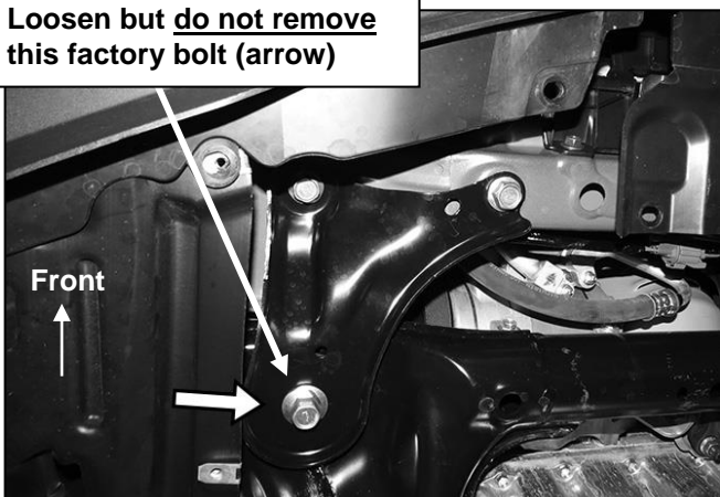
(Fig 5) Passenger/right side pictured from below. Temporarily loosen the factory bolt (arrow)
