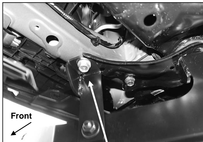
(Fig 4) Reuse factory hex bolt to attach passenger/right Support Bracket to cross member
