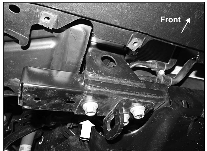
(Fig 2) Remove factory hex bolt (arrow)
